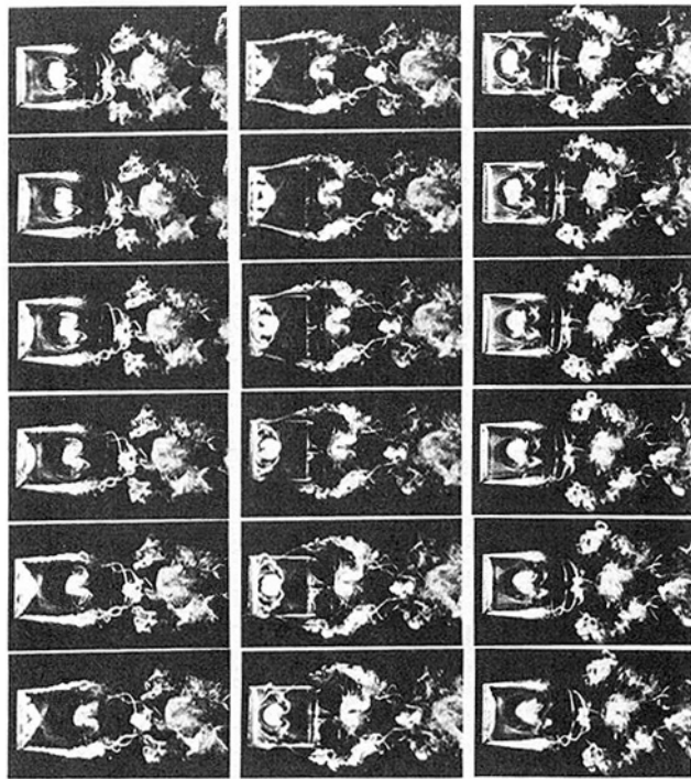
Fig. 7 Square wing in periodic pitch from 0 to 30 deg, f=2\text{Hz} , c=15\text{ cm} , U_0=61\text{ cm/s} , R=5100 , \Delta t=1/32\text{ s} . Remarks: \alpha=30\text{ deg} in frame 3, column 1; \alpha=0\text{ deg} in frame 5, column 2; the last 2 frames of column 3 are part of the next cycle.
